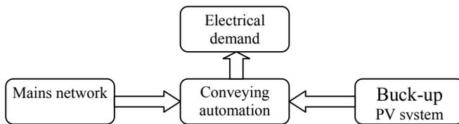
Figure 1. Schematic of a back-up powering system.
