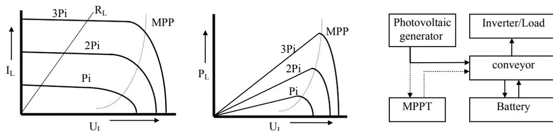
Figure 2. Power as a function of voltage and the schematic of a Photovoltaic system
